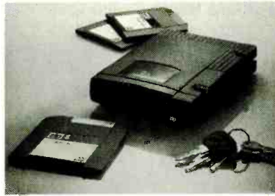
Fig. 1. Iomega's Zip floppy-based drive is today's market leader. This 1.44MB look-alike provides 100MB at low cost, and is the most likely replacement for the venerable floppy.
